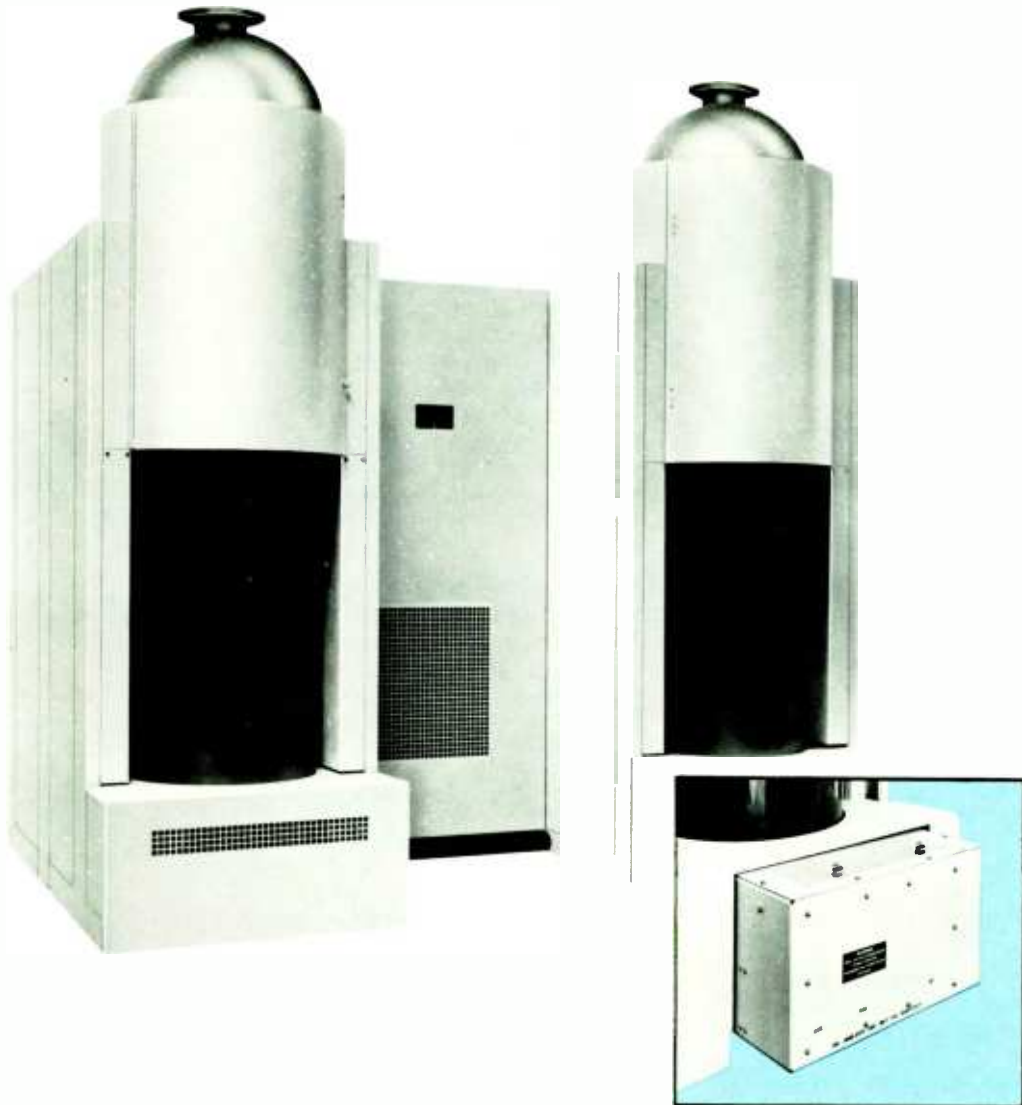
TVE-30, rear view. (Inset) Mod Anode Pulsar.
