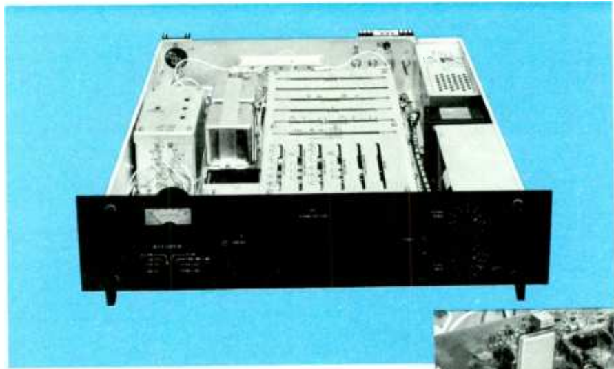
The MCP-1V visual exciter/modulator is a solid-state, independent, self-contained "on-channel" signal source. Harris' TSB filter (right) is mounted on a PC board in the visual exciter, and measures only 1½ inches square.
