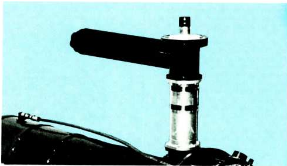
The Variable Visual Coupler employed in the TVE-55 greatly increases the visual klystron's efficiency over the previously used fixed couplers.
